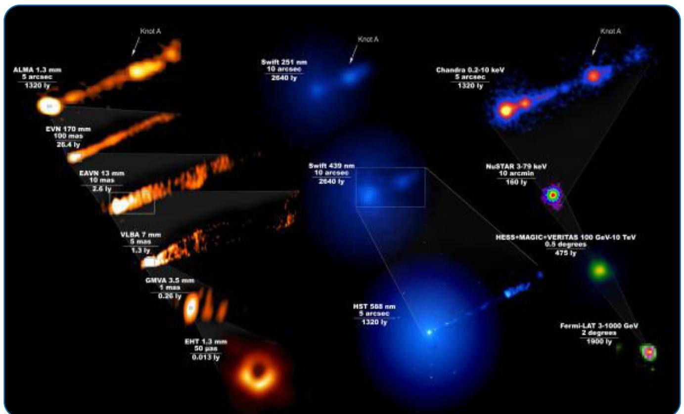
*Compilation of the quasi-simultaneous M87 jet images at various scales during the 2017 campaign. The instrument, observing wavelength, and scale are shown on the top-left side of each image. Note that the color scale has been chosen to highlight the observed features for each scale, and should not be used for rms or flux density calculation purposes. Location of the Knot A (far beyond the core and HST-1) is shown in the top figures for visual aid.*
