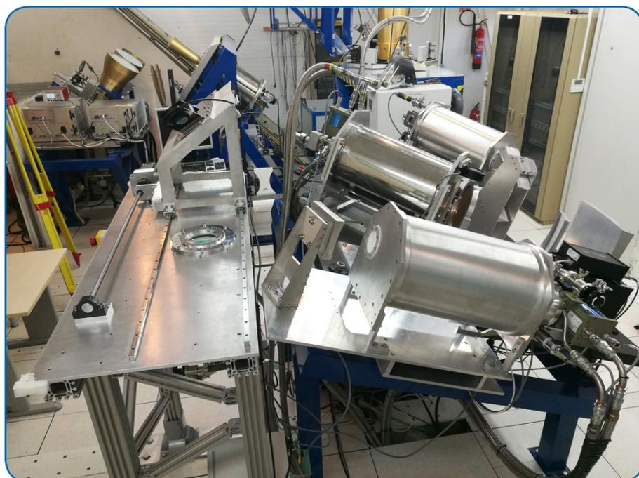
*The high frequency receivers at the 40m RT receiver cabin. On the left, the hot and cold calibration system. The W band receiver is the one closer to the observer. The farther one is the Q band receiver and in between both, the K band one is located.*
