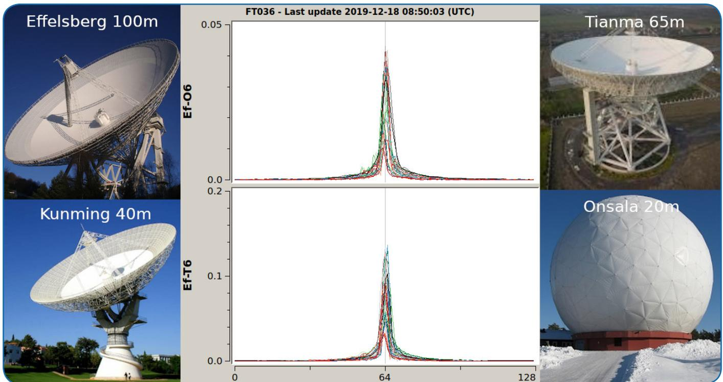
*Fringes between the stations Effelsberg (Ef), Onsala (O6), and Tianma65 (T6) together with pictures of all stations involved in the test. Note that there are no fringes to Kunming due to a recorder failure at the station.*
