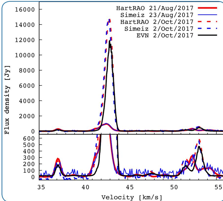
*The scalar averaged, cross-power water maser spectrum measured with the EVN (solid, black line) is shown in comparison to single-dish spectra provided by the M2O on the same date (dashed red and blue lines), and (solid red and blue lines) pre-flare. The panel below highlights the low-flux density maser features.*
