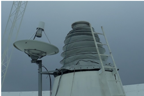
Figure 5.19: The new uncooled L-band receiver – feed antenna at RT-32 secondary focus (left) and IF unit (right)
