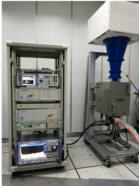
Figure 5.20: The new C band receiver tested in laboratory.
