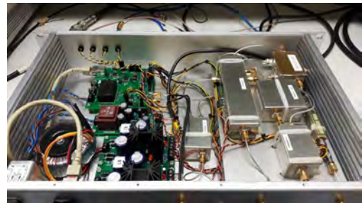
Figure 5.19: The new uncooled L-band receiver – feed antenna at RT-32 secondary focus (left) and IF unit (right)
