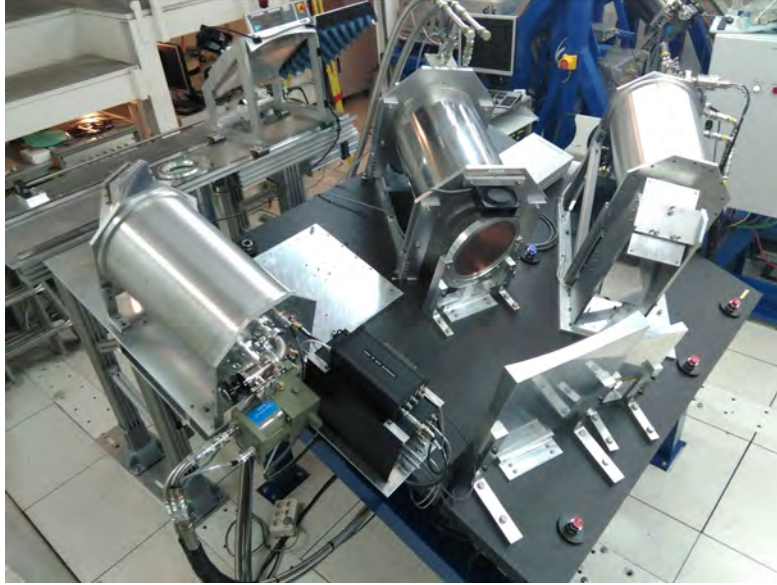
Figure 5.10: Optical table with 3 receivers, 22, 43 and 86 GHz. By the time of the report 22 and 43 GHz can be used simultaneously.
