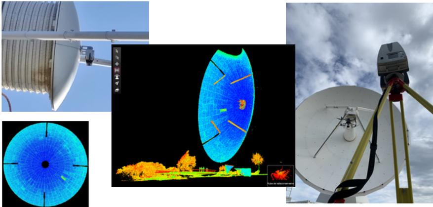
**Figure 5.5:** Laser scanner and drone surface measurements for RT40 and RT13.
