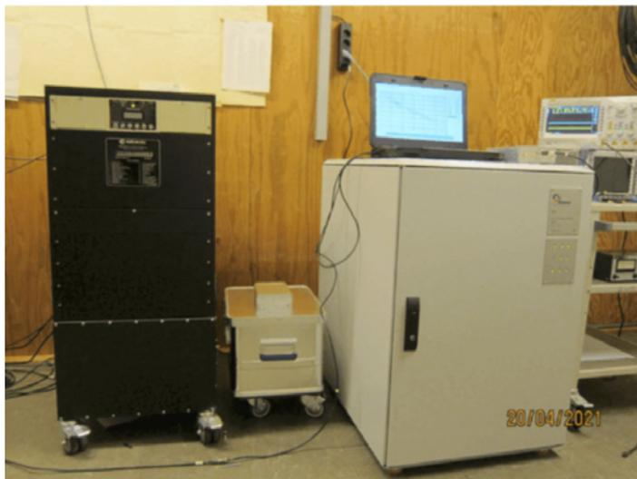
**Figure 5.1:** The old MASER (left), which was almost 25 years old, next to the new MASER (right) of the WSRT, which was installed in April 2021.
