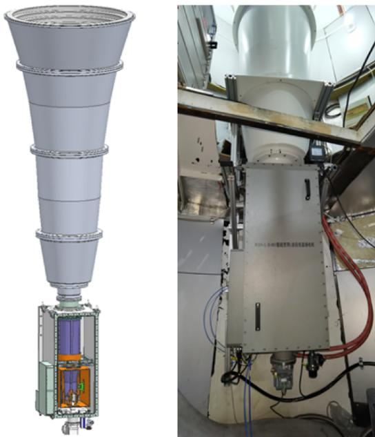
**Figure 5.13:** The simulated picture (left) and installation status (right) of the new L-band receiver.
