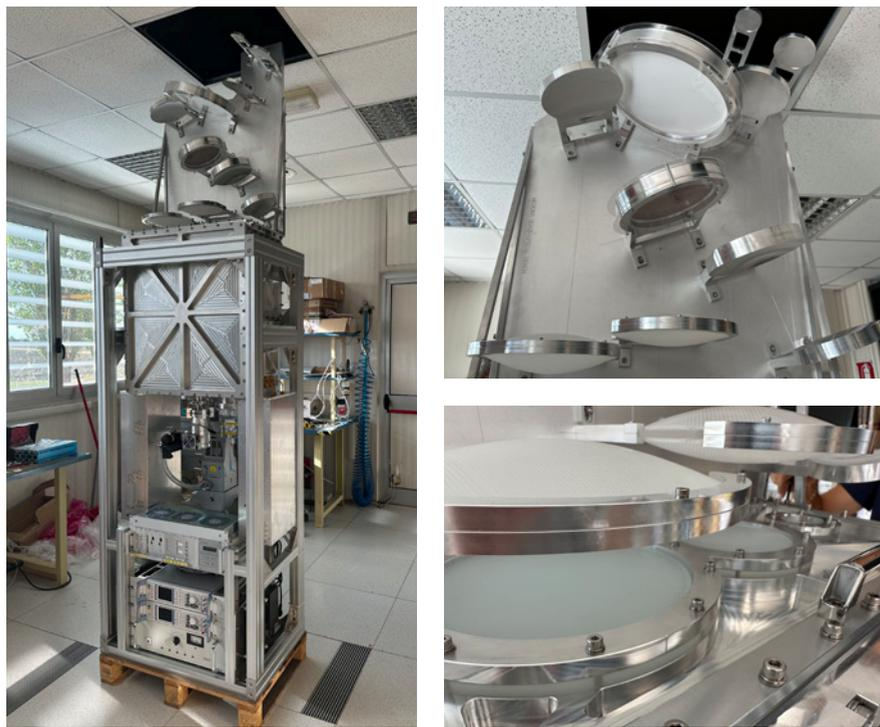
**Figure 5.2:** Images of the Compact Tri-Band (CTR) receiver at the Medicina radioastronomical station. Left: Complete CTR to be mounted on Medicina and Noto antennas. Right: views of the quasi optic system providing the frequency simultaneity. A similar system was also acquired for installation on the Sardinia radio telescope.
