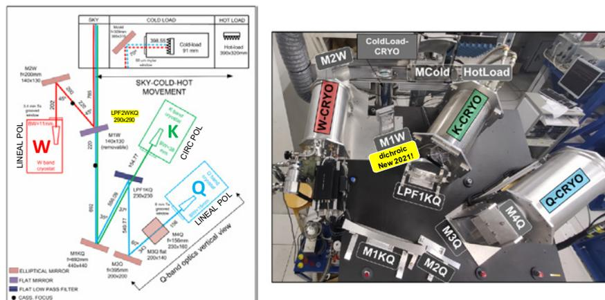
Figure 5.4: Optical components and signal path for VLBI observations in K-Q-W bands simultaneous reception.
