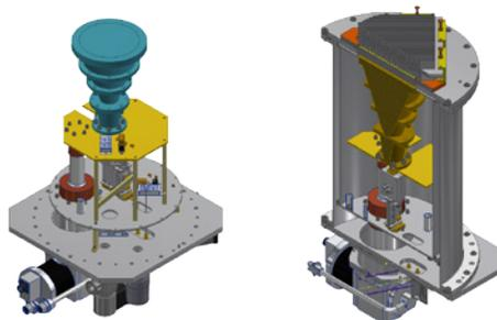
Figure 5.3: New ASTROREC K-band receiver under development.
